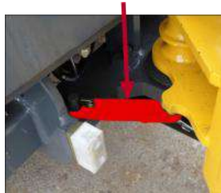
Articulated joint blocked
