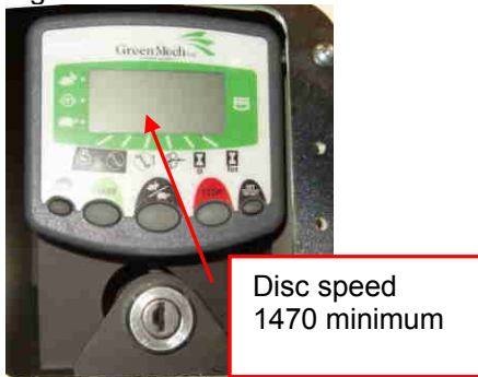
Fig 5.7.2 RDS Control unit
